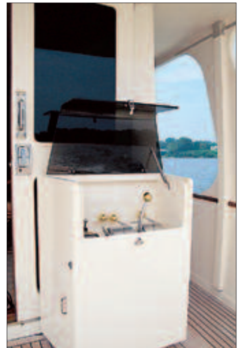
Aft control console house engine controls, thruster control, and autopilot remote.
