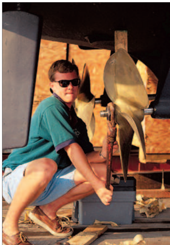
Mick Shove tightens up 5-bladed delivery props. The boat will be fitted with 4-bladed props back at the Burr Yard.
